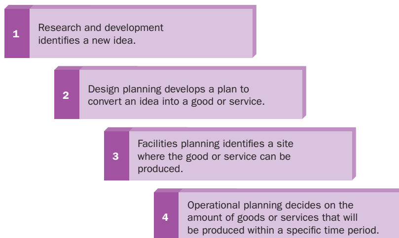
FIGURE 8.3: Planning for Production Once research and development have identified an idea that meets customer needs, manufacturers use three phases to convert the idea to an actual product or service.
